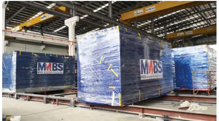
The 3D units are transported and erected on-site in less than a couple of days
